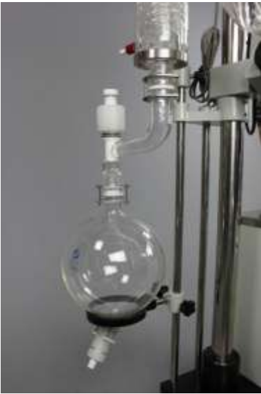
连续收集 - 单收集瓶 Non-stop Receiving by One Flask
