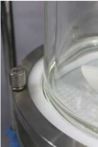
夹套全覆盖，保温效果显著 确保滤液不结晶 Full Jacket for Insulated Filtration against Crystallization
